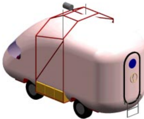
Figure 4. A rear view of the HOP. The vehicle will include a simulated airlock.
