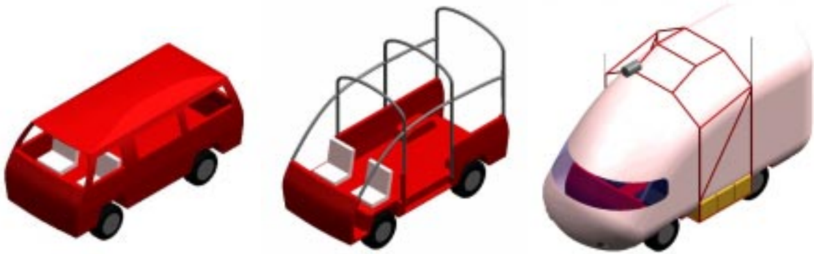
Figures 1-3. The HOP; from the base vehicle to the final structure.
